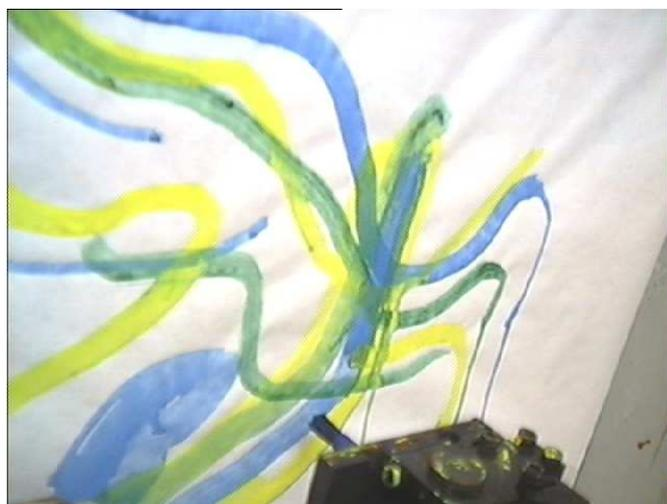
**Figure 4 Camera 1 view of the easel, the robot end effector, and the tip of the paintbrush. (Wilkes site)**
